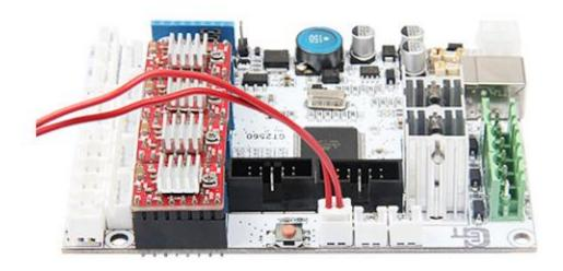
2) Connect wires for thermistor of extruder 1.
