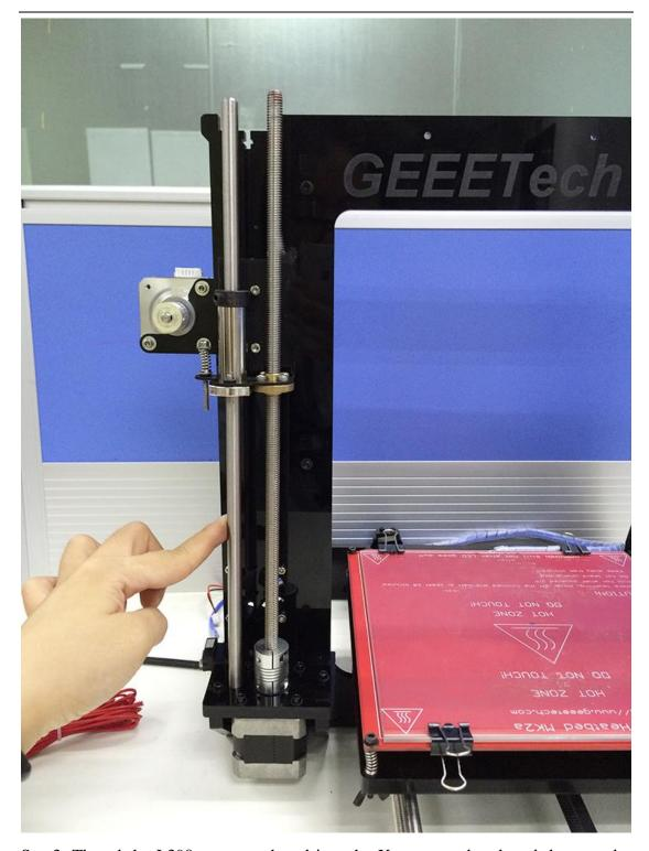
Step3. Thread the L390mm smooth rod into the X motor end > thread the extruder carriage on the two rods.
