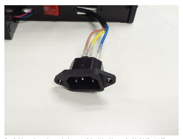
Step2. Mount the socket on the bottom of the right side panel with 2 M3 x 16 Hex Counter- sunk-head screws and M3 hex nut.
