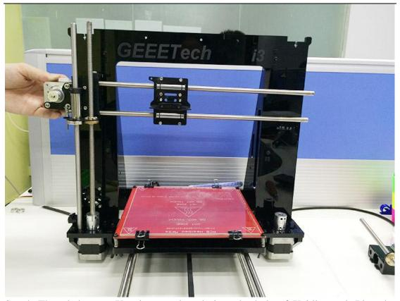
Step4. Thread the two X axis smooth rods into the hole of X idler end. Plug the vertical trapezoidal screw into the coupling on the right bottom of the Z axis. Then thread the 320mm smooth rod into the linear bearing.
