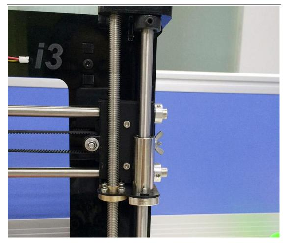
\*Note the direction of the driven wheel, the side with bolt head should be towards the A1, or it will scratch the acrylic plate.
