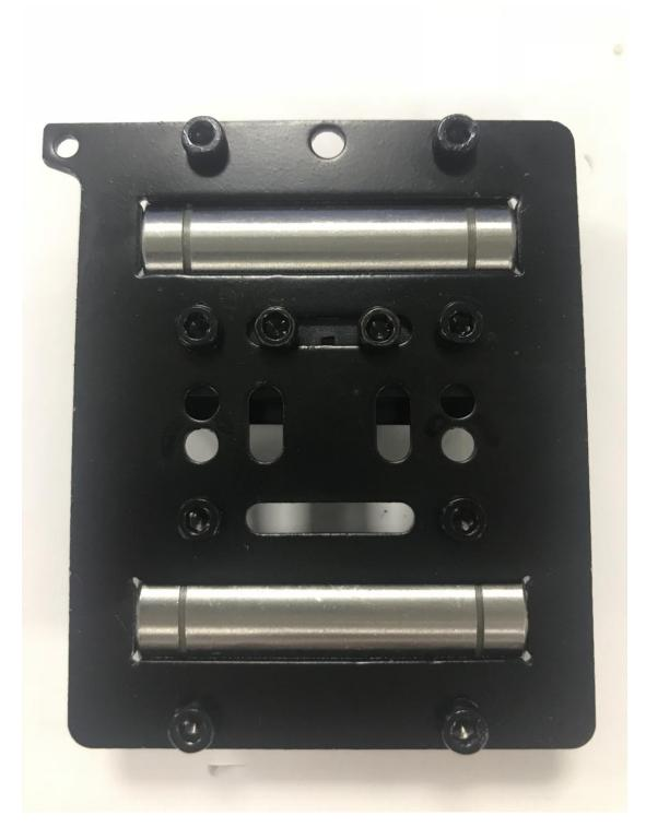
Step3. Fix the extruder holder on the front side of the X carriage using M4x6mm screws.
