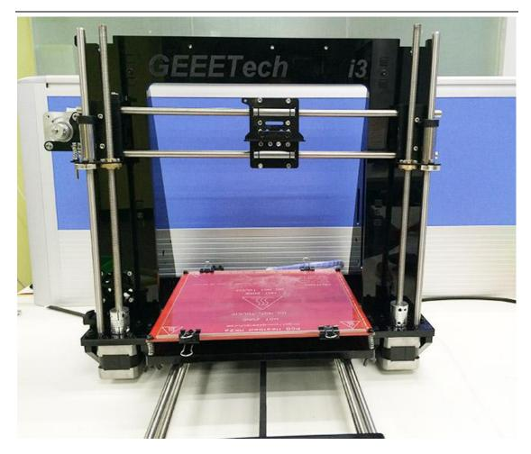
Note: the smooth rods and the trapezoidal screw of Z axis are vertical and the X axis is horizontal, which is very important, or it will hinder the move of the Z axis.
