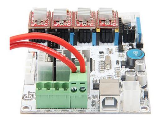
2) Connect heating wires for extruder 1.
